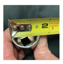
Find a socket that measures between 1 7/16" and 1 1/2" (1.4"-1.5"). Size should be confirmed by measuring using a tape measure.
