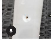
5. Using small wood screws, countersink holes into the PVC and insert two small wood screws
