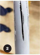
2. With a handheld angle grinder and a cut blade, cut longitudinal vent openings
