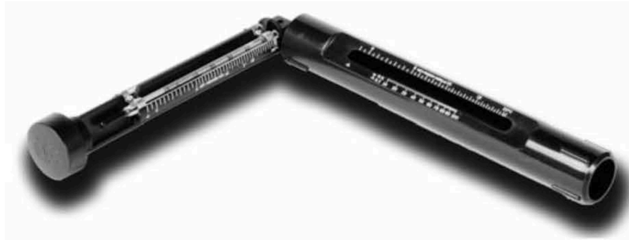
Figure 4. A photo of a sling psychrometer
